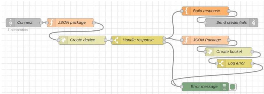
Fig. 2 - Node registration implementation in Node-RED.
