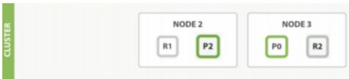
Cluster after killing one node. Elasticsearch: The Definitive Guide. Clinton Gormley, Zachary Tong. 2011
