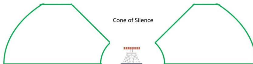
Fig.2: Vertical-Central Section of the Coverage Volume (not to scale).
