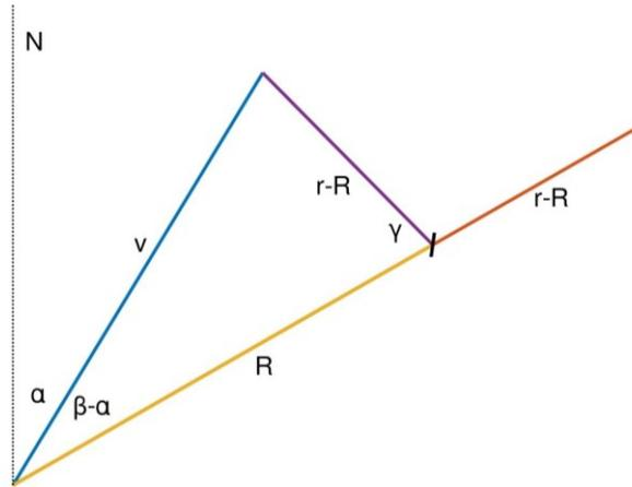
Fig.6: Geometry for calculating the Location of the Reflector.
