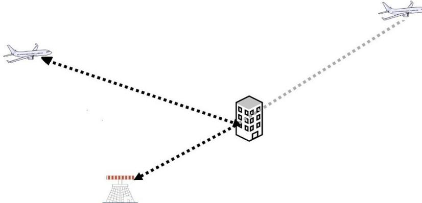
Fig.5: Geometry of Reflections
