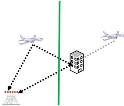
Fig.7: Singular Case of Geometry of Reflections.
